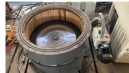
Maglev Overspeed Test Bench 磁悬浮叶轮超速测试台
